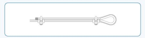
step2. The second wire rope clip must be placed immediately against the thimble but nevertheless in such a position that correct tightening of the grip does not damage the outer wires of the rope. The second clip is fastened with a force equal to or less than a specified torque to be fastened to each other.
