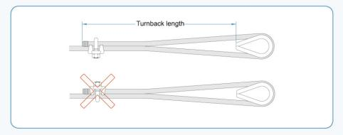
step1. The first clip must be placed one saddle width from the turned back rope tail or dead end of the rope. U-bolt is fastened toward the dead-end direction of the rope. The first clip is fastened with the specified torque.
